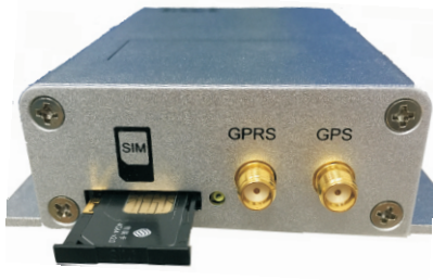
Fig 4 SIM card diagram for IP20 model
